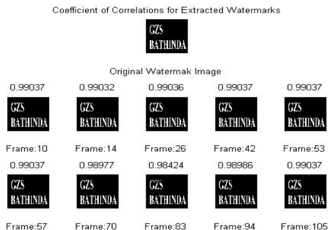
Fig. 3: Original watermark, extracted watermarks from all the 10 watermarked frames with frame number & their correlation factors
